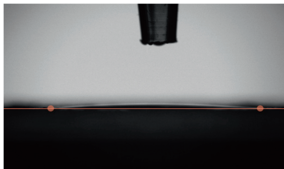
Fig. 3. Contact angle of SiO 2 nanoparticles dispersion solution.
